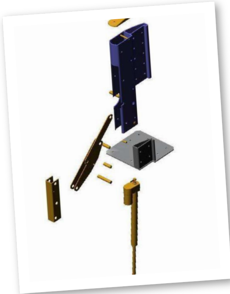
Lift Gate design for Maxon Lift. Consumer truck application. Exploded view, one side of actuator system.
